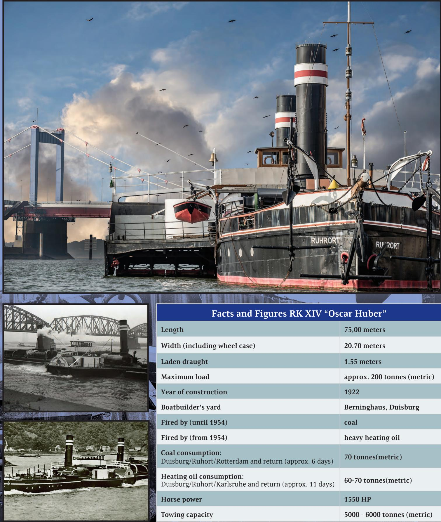
the original coal-firing tug was converted to oil.
