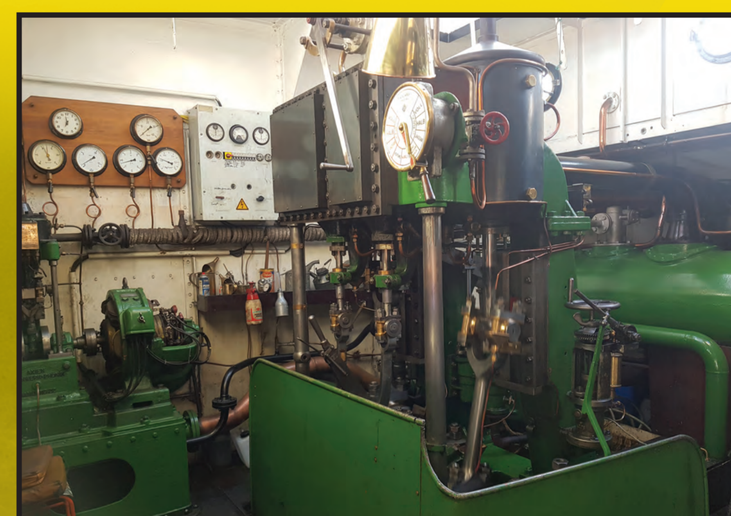
2-Zylinder vertical steam engine, 280 PSI
